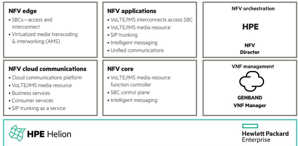
GENBAND SBC VNFs, for example, allow CSPs to independently scale control or signaling and media planes for customer-facing services. Along with the standards-based GENBAND VNF Manager, operators can scale services up or down—on demand or automatically—entirely through software. They can integrate the speed and scale of **NFV** into their existing hybrid networks, orchestrating both virtual and physical resources to create customized service offerings.
