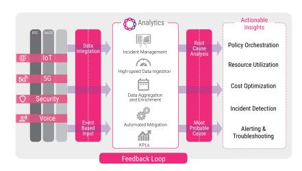
**Multi-access Edge Computing (MEC):** Autonomous systems allow traffic classification at the network edge, allowing traffic streams requiring real-time processing to be allocated to MEC resources and those not requiring local processing to be allocated to the core for processing.
