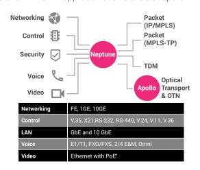
Traditionally, TDM provides the tools to derive and distribute accurate timing, which is fundamental to maintaining the operation of the monitoring and control devices. As networks evolve to packet, the timing architecture must remain robust. The solution allows an approach similar to that used in TDM. A built-in GPS receiver or an external timing source provides the master clock. 1588v2 Precision Timing Protocol (PTP) distributes timing across the network
