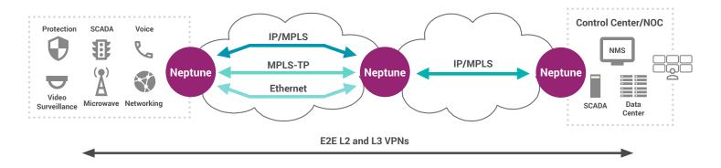
In addition to standard L3 VPNs (using E2E IP/MPLS) and L2 VPNs (either using static MPLS-TP or dynamic IP/MPLS), Elastic MPLS offers additional advantages, including:
