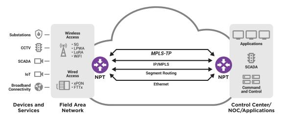
In addition to standard L3 VPNs (using E2E IP/MPLS) and L2 VPNs (either using static MPLS-TP or dynamic IP/MPLS), Multi-stack MPLS offers additional advantages, including:
