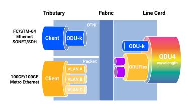
(new services added, changing service locations), because it leverages the common network resources as efficiently as possible. Rather than requiring all encapsulated services to be terminated at the same point, OTN switching allows individual services to be extracted from the larger container and added/dropped flexibly at intermediate sites. This capability ensures that the network wavelengths remain as fully utilized as possible, even on a network with a variety of demands at multiple sites.
