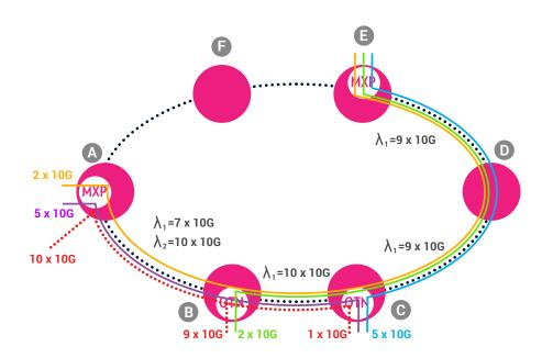
With expandable OTN, the two sites with OTN switches can be built using just enough switching capacity to support the traffic requirements. If more demand is added to the network – either a new customer or an expansion of demand from an existing customer – additional OTN switching can be added as needed, easily and economically.
