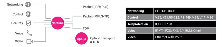
As networks evolve to packet, the deterministic, bidirectional traffic paths used by MPLS-TP ensure that robust timing is maintained. For critical infrastructures wishing to use their unique geographical footprint to generate extra revenues as a Utelco, the multiservice capabilities of Neptune provide the managed L2 and L3 VPNs required for business services, residential services, mobile backhaul, and future IoT applications. Muse LightSOFT provides network management for all
