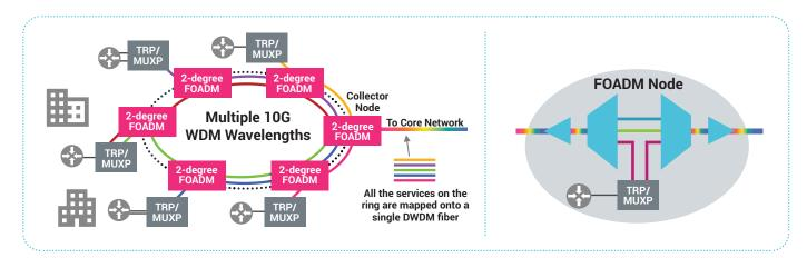
However, a new generation of economical Small Form Factor OTN switches, like the Apollo 9901X, is starting to change the equation, particularly for Layer 1 business services. These enable the ring to use a single 100G wavelength rather than a WDM fiber. Services connect to the OTN switches via low-cost gray interfaces, and are added to the ring traffic under software control.
