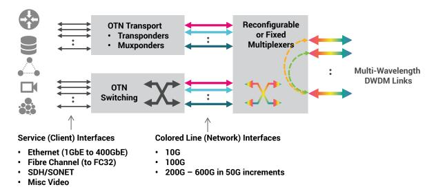
The first step relies on the Optical Transport Network or OTN technology. This standard structure encapsulates one or more services into different sizes of optical containers and adds bits for error correction and operational monitoring. OTN then modulates the resulting bitstream of service payloads plus overhead onto a colored wavelength. In optical networking systems, OTN technology is implemented in two practical ways:
