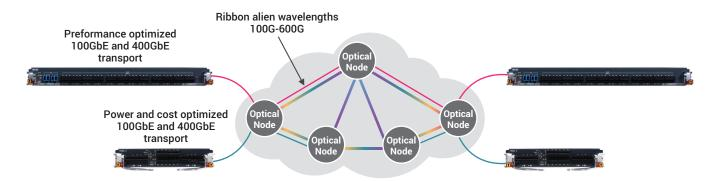
Ribbon enables RENs to overcome this challenge by deploying Apollo optical transport solutions over the existing infrastructure as alien wavelengths, including over brownfield fixed grid 50GHz and 100GHz spacing networks. This enables taking advantage of the many performance and economic benefits Apollo transport brings without a forklift upgrade. Apollo's transport blades cover all application spaces. All Apollo transport blades are controllable through standard OpenConfig APIs.
