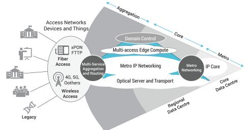
The solution is intelligent use of optical networking seamlessly integrated with an IP networking layer that supports deterministic IP networking. In this approach, high-bandwidth services are handled directly by the optical layer, while lower bandwidth services are aggregated at the edge of the network and then transported across the network using the most appropriate networking technology to meet their performance characteristics.
