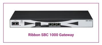
The Ribbon SBC 1000 Gateway is an entry-level solution for Voice over IP connectivity and security: a base model that can be expanded through hardware and software upgrades to meet the needs of growing companies like PIVOT. It can connect legacy telephony endpoints to emerging technologies like Teams, allowing PIVOT to migrate to Teams calling at their own pace with no change in hardware or licensing.
