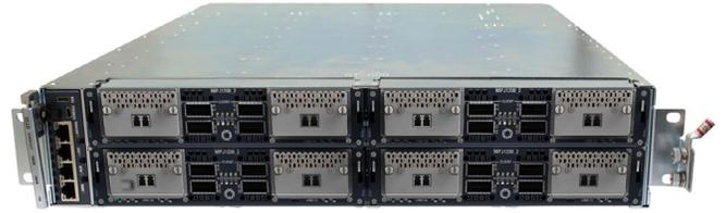
Apollo 9408 is the industry's highest capacity and highest density platform for 100GbE, 400GbE, and future 800GbE transport. It is designed to provide network operators with the lowest cost per bit for long haul and high traffic density metro applications.
