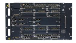
The powerful Elastic MPLS engine provides future-proof evolution with converged support for MPLS (IP and TP), Ethernet (MEF CE2.0 certified), segment routing, and TDM over CES/CEP. OTN mapping and WDM interfaces allow seamless hand-off for bulk optical transport.
