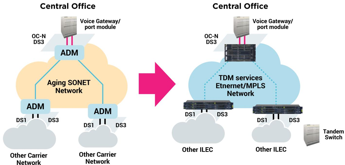
The new IP/MPLS network uses standards based circuit emulation (CES) approaches (SAToP and CESoPSN) to enable it to support all of the functionality required to provide voice trunks:
