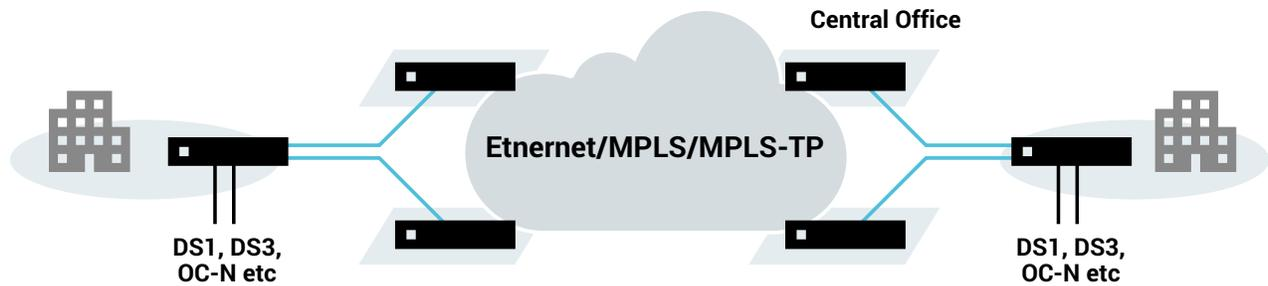
As mentioned previously, the packet network uses circuit emulation to provide enterprises with a reliable platform for supporting their legacy SONET services. Direct DS1, DS3, OC-3/12 interfaces allow existing services to be directly connected to this packet network.
