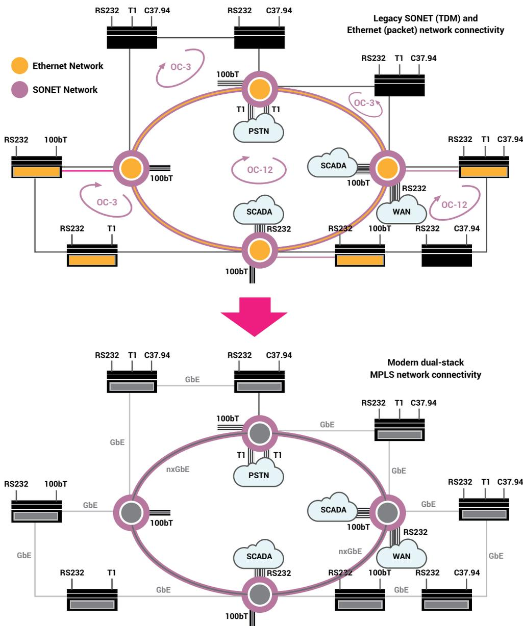
In the legacy network, specialized SONET equipment designed to carry SCADA and other TDM traffic including T1, RS232, and C37.94 Tele-protection traffic. At interconnection points, ports on the SONET equipment is reserved to route traffic between rings. A packet network carries Ethernet traffic for the IT services.
