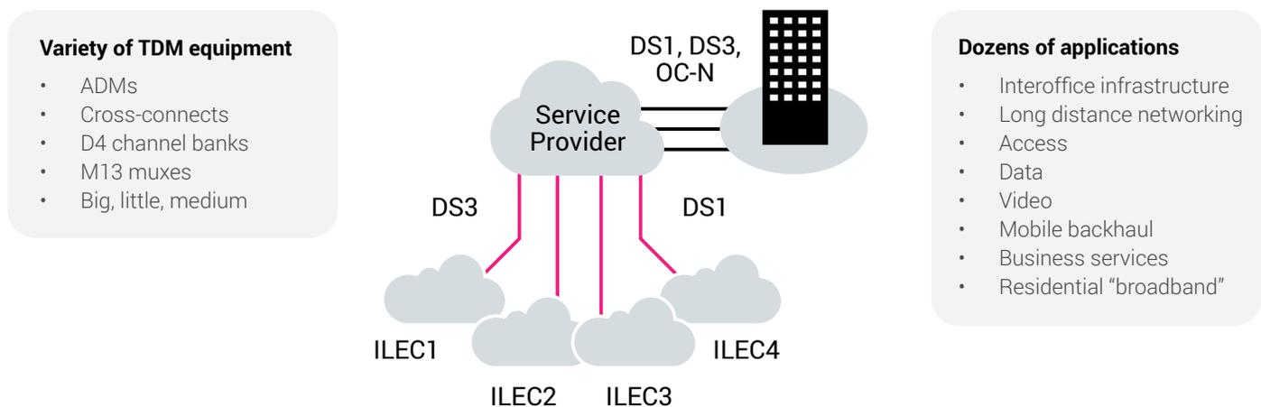
Service providers already have established packet networks to support IP and Ethernet services. However, most of these Service Providers are also running a TDM network in parallel to the packet network. This legacy TDM network enables them to continue to support customers with high-value legacy SONET services such as private line services or support legacy infrastructure like voice trunking.
